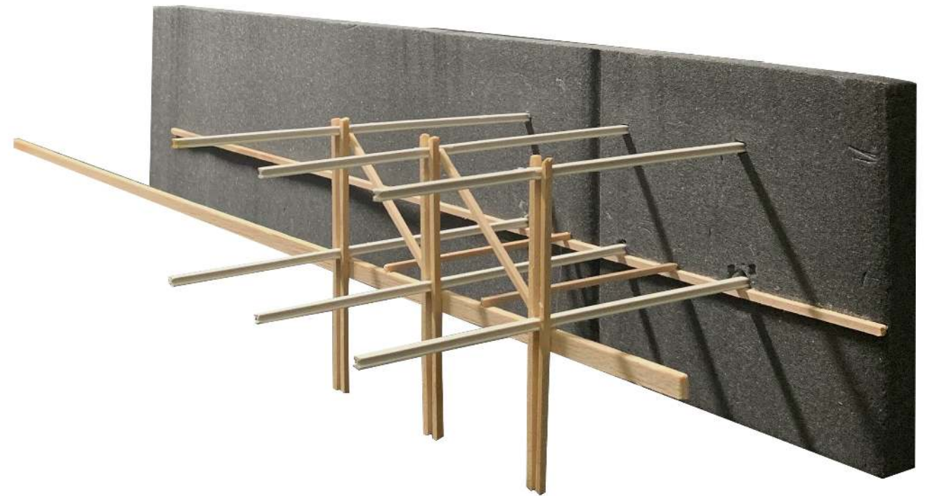
1:50 Structural Model of Frame Connection to Gabion
